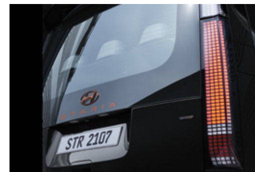
Parametric pixel lights (LED rear combination lamp)
