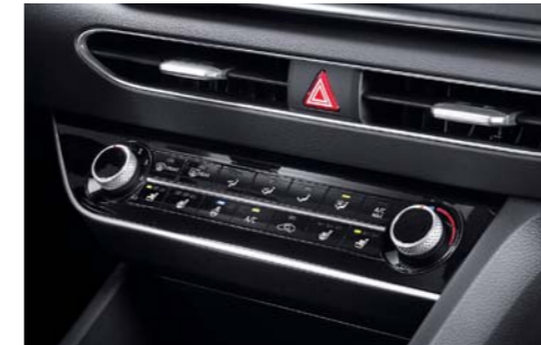
Manual air conditioning system
